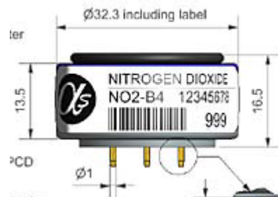
Figure 19: Dimension of the \text{NO}_2 -B4 sensor
