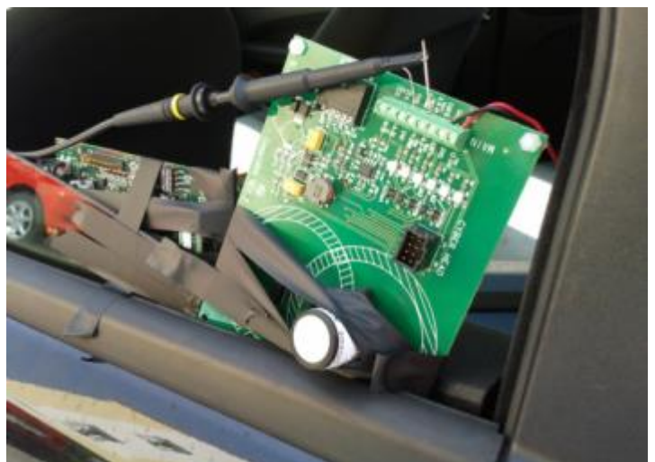
Figure 23: Installation of sensors for the first pre-measurement campaign
