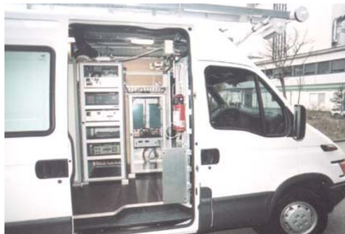
Figure 13: Racks for gas phase measurements (left rack) and power supply (right rack) 4
