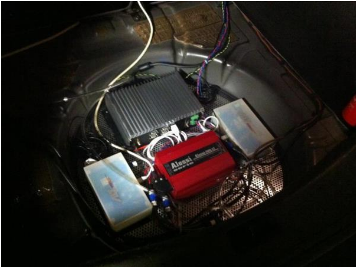
Figure 2: Integration of the on-board units in the AIT demo vehicle
