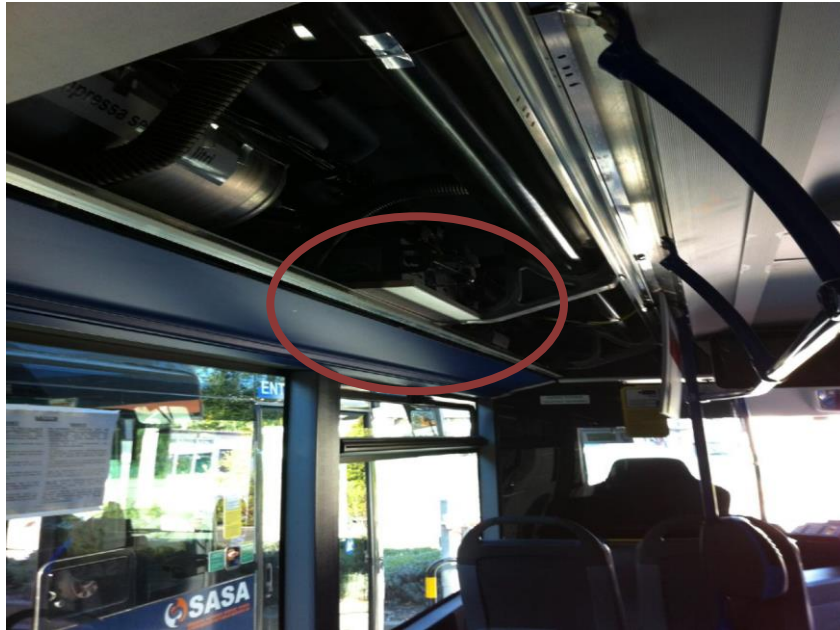
Figure 19: Mounting place of the Mobile System in the SASA bus
