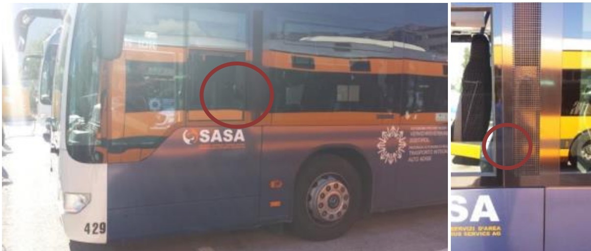
Figure 20: Position of air tube in the SAS-bus
