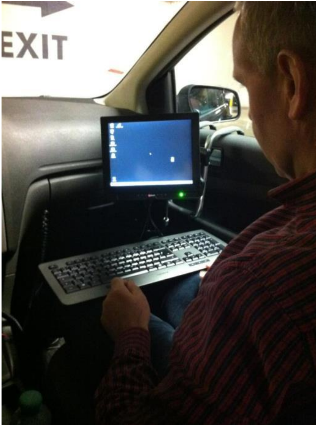
Figure 4: Integration of the operator HMI in the demo vehicle.
