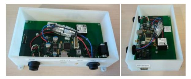
Figure 12: Traffic monitoring unit without cover
