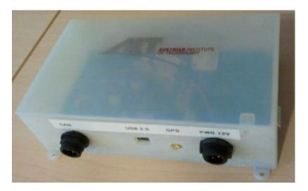
Figure 11: Traffic monitoring unit prototype
